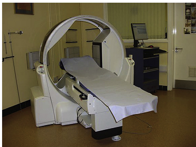
Figure 1 Sodium iodide gamma camera designed for dedicated cardiac work. The sodium iodide crystal heads lie perpendicular to each other and rotate around the patient's heart in 32 steps. Collimators in front of the heads allow only perpendicular photons through to the crystals. The resulting scintillation is amplified by photomultiplier tubes and converted to an electrical signal that is gated to the patient's ECG. Trans-axial slices are created, reconstructed to standard orthogonal planes and displayed on the computer workstation. Fixed planar imaging (non-rotating camera heads) is no longer used for MPS work; SPECT is preferred, especially as it allows functional assessment.
