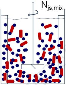
Modified power model: •Non-spherical particles •Networking effect •Up to 55 wt% solids
