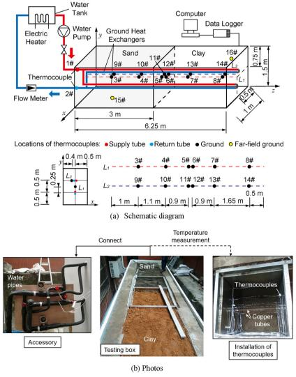
Fig. 1. (a) Schematic diagram and (b) Photos of the experimental rig used in this study.
