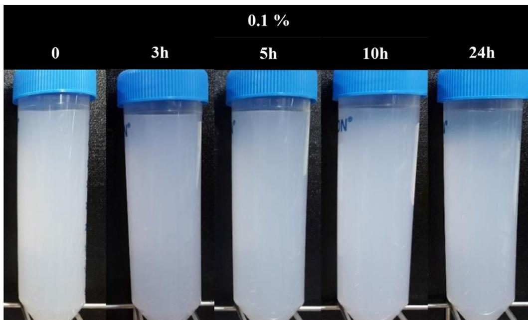
Fig. 1. Photographs of  $\text{Al}_2\text{O}_3$  nanofluids at various times.
