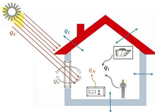
**Fig. 1.** Heat exchange mechanisms between an indoor space and its external environment. Solar radiation ( $Q_s$ ) and internal heat sources ( $Q_i$ ) i.e., occupant body, light fixture, etc. only contribute to the heat gain of the space. On the other hand, convection ( $Q_c$ ) through roof, walls, and floor, ventilation ( $Q_v$ ) through open windows and doors, and mechanical heat sources ( $Q_m$ ) i.e., HVAC unit, space heater, etc. can contribute to either heat gain or heat loss.
