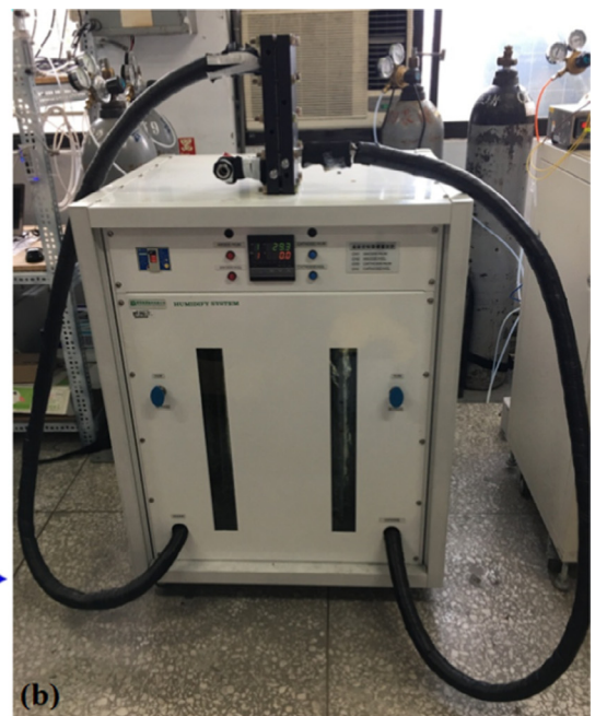
Fig. 1. (a) The test setup used for the humidification practice; (b) The photo of the test setup.
