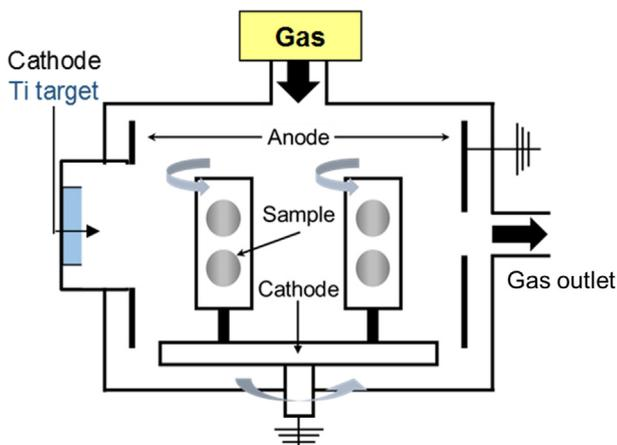
Fig. 1. Schematic of the PECVD and PVD apparatus.
