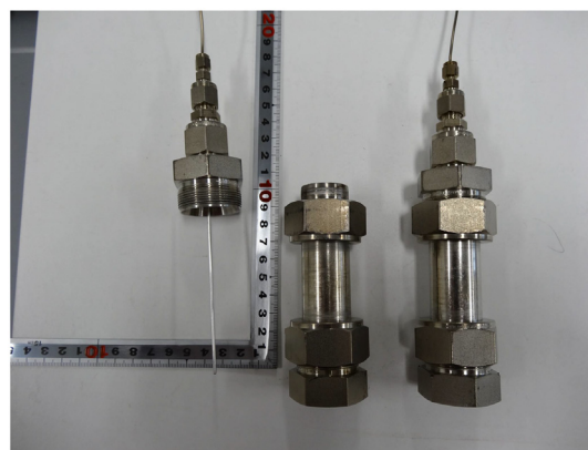
Fig. 1. Tube reactors used for hydrothermal pretreatment. Approximate dimensions: outer diameter, 25.4 mm (1 in.); wall thickness, 1.65 mm; length, 100 mm; and inner volume, 38.0 mL.
