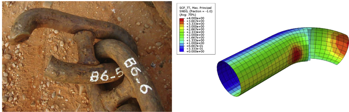
Fig. 1. Cracked mooring chain and stress distribution on the chain surface under tension.
