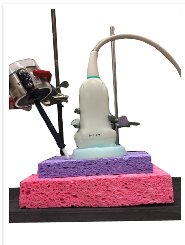
Fig. 1. Experimental setup. An ultrasound probe was placed atop an ultrasound gel pad to measure the surface wave speed of the lung phantom—the purple sponge. The pink sponge and the black rubber were placed under the purple sponge to reduce the reflection of the sound wave from harder surfaces. A shaker was in contact with the purple sponge surface to generate harmonic vibrations on the sponge surface. The bars behind the shaker and the ultrasound probe are the holder frames used to keep the equipment in place.
