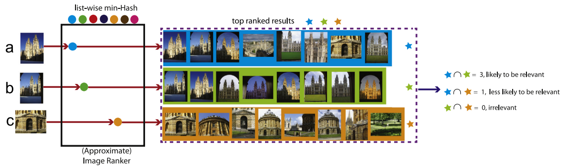
Fig. 1. Ranking consistency overview. The examples are top ranked results of all souls 1 , where the input image A and B are relevant, but both of them are irrelevant to C. Our method generates some top ranked results for each image by list-wise min-Hash. The similarity between images is measured by the similarity between their top ranked results.
