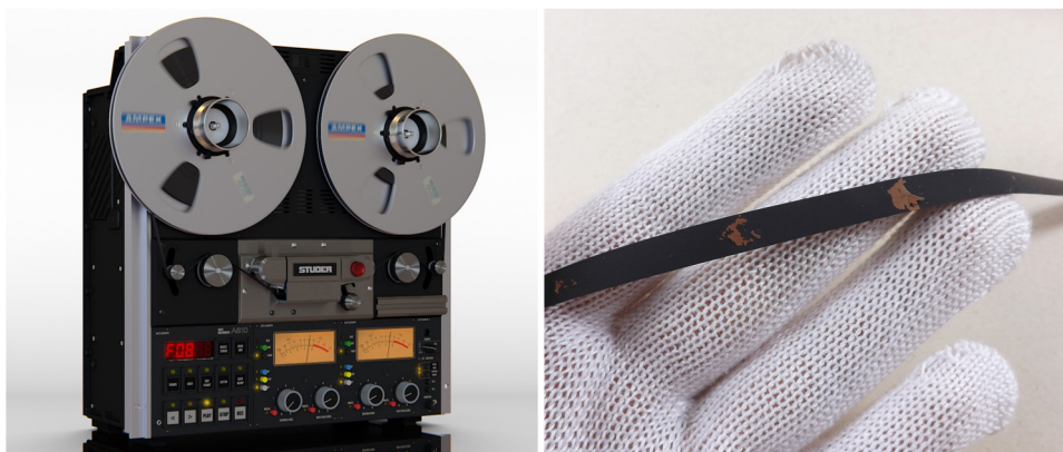
Fig. 1. Left: open reel tape on a stereo recorder. The tape is 1/4 inch wide, and its average transfer speed is 9,5 cm/s or 19 cm/s. Tapes are usually wound on metal or plastic reels. Right: close-up on a damaged tape. Small portions of the magnetic side of the tape (light brown) came off and remained attached to the back of the tape (black).
