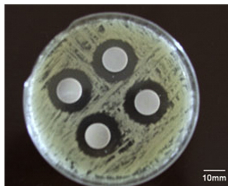
Figure 1. Photograph of antibacterial test results of AgHA-IE samples against E. coli . 28 Reprinted from applied surface science, 257, Stanic V., Janackovic D., Dimitrijevic S., Tanaskovic S. B., Mitric M., Pavlovic M. S., Krstic A., Jovanovic D., Raicevic S., Synthesis of antimicrobial monophasic silver-doped hydroxyapatite nanopowders for bone tissue engineering, p. 4510, Copyright (2011), with permission from Elsevier.
