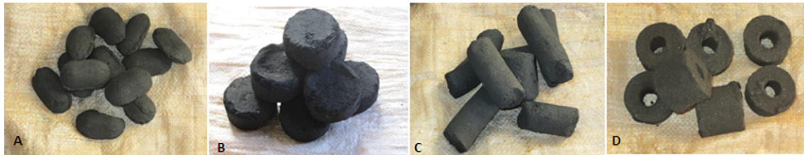
Fig. 1. Carbonized briquettes on the market. A – Pillow Carbonized charcoal dust briquettes; B – Cylindrical char dust briquettes; C – Pelleted char dust briquettes; D – Hollow carbonized saw dust briquettes. It is important to note that differences due to briquette composition or materials used and tree's species from which charcoal was made were not analyzed for as the vendors could not be in position to tell what materials the briquette supplier used or what tree species the charcoal supplier used. It was not also possible to get briquettes of the same size and shape from different manufacturers and this informed the choice of the nested design used. However, the researcher was able to establish that majority of briquette manufacturers use matooke peels as one of the main materials from those who supply the peels to them after gathering them from garbage sites to earn a living shown in Fig. 2.
