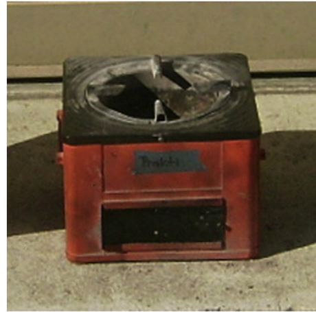
Fig. 3. Prakti rouj stove: height: 20.5 cm; diameter: 25.5 cm; weight: 4.6 kg.
