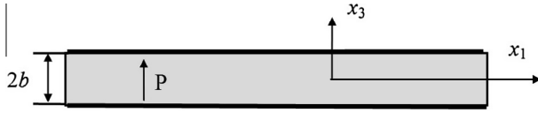
Fig. 1. A piezoelectric plate and coordinate system.
