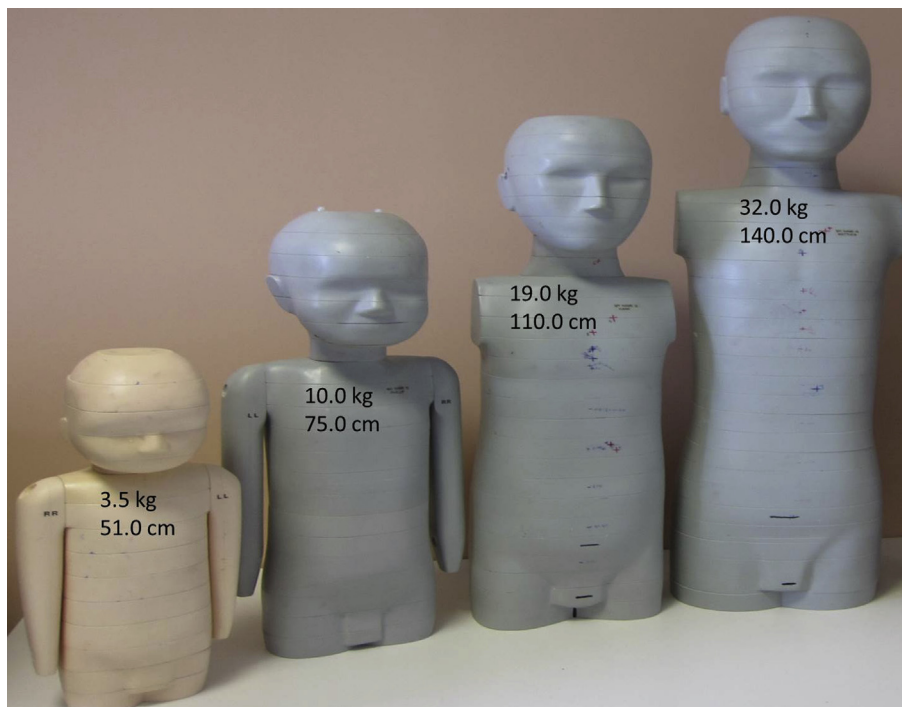
Figure 1. Pediatric anthropomorphic phantoms representing the average individual as newborn, 1-year-old, 5-year-old and 10-year-old child, from left to right. Data on their weights (kg) and heights (cm) are displayed for each phantom.
