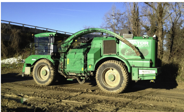
Fig. 1. The Albach Silvator 2000 agro-forestry chipper used in the study.
