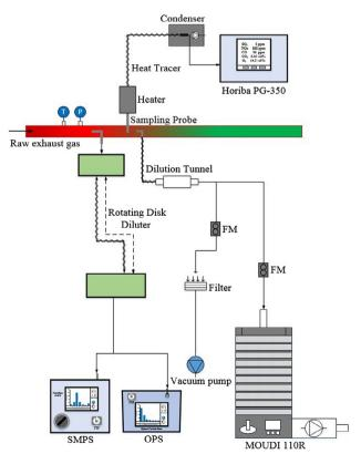
Fig. 1. Schematic diagram of marine diesel engines exhaust emissions test setup.
