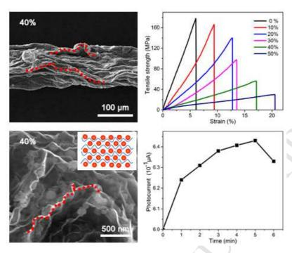
Stretchable conductive graphene fibers with highly wrinkled architecture, which are fabricated by the uniform intercalation of TiO<sub>2</sub> nanoparticles between graphene sheets via a simple wet spinning technique, show high breaking elongation and excellent photoelectric properties.
