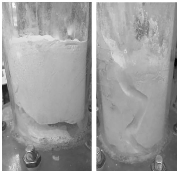
Fig. 3. Slugs and channels at the LiF fluidization process.
