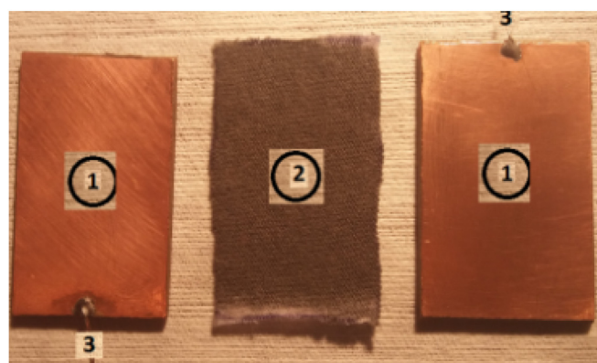
Fig. 2. The components of the flat capacitor (FC): 1 - Copper plate; 2 - Active magnetic fabric (AMF).
