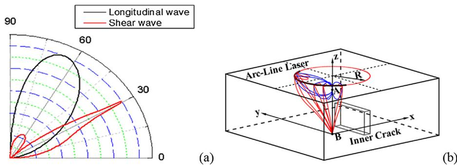
Fig. 1. The relationship between the focal points of bulk waves and the shape of arc-line laser source: (a) directivity of bulk waves in thermoelastic mode, (b) schematic of the convergence of bulk waves generated by the arc-line laser.
