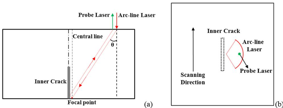
Fig. 2. Schematic diagram of inner crack inspection with arc-line laser: (a) cross-section view and (b) top view.
