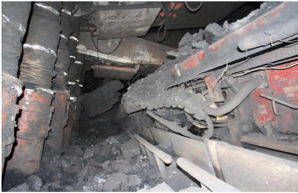
Fig. 1. Results of coal burst in longwall working face (Lu et al., 2015).
