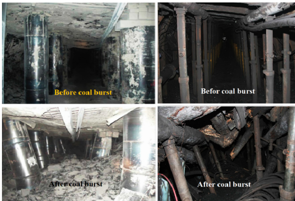
Fig. 2. Coal burst effects on mine working space (Wang et al., 2016a; Christopher, 2016).
