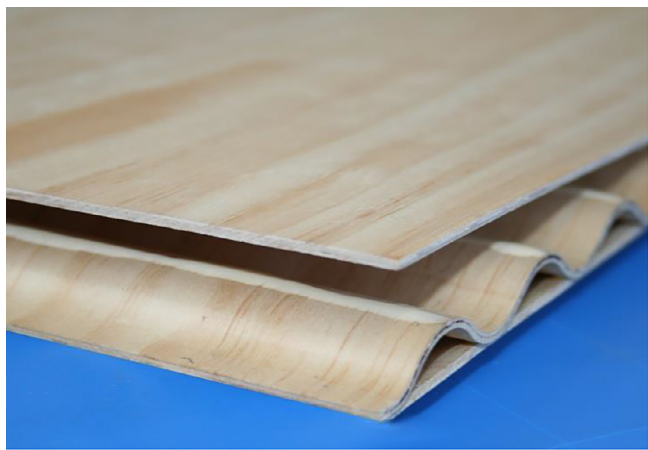
Fig. 1. Bonding the core to face-sheets. Consistent lines of adhesive were applied to the corrugation peaks, then face-sheets were assembled and held in place as the adhesive set.
