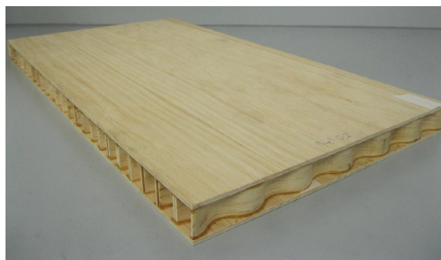
Fig. 2. A panel manufactured with sinusoidal honeycomb core, which was not the focus of this study, but has promising properties.
