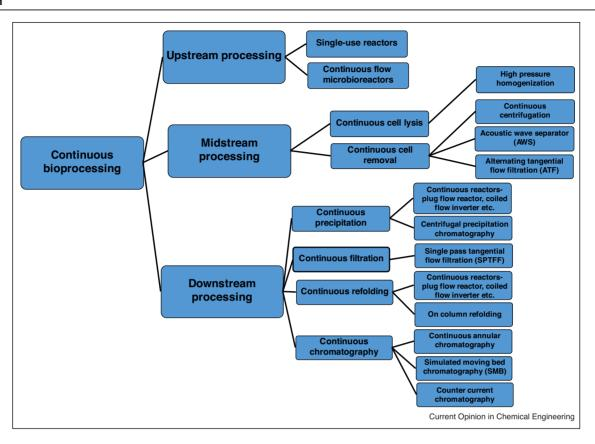
Schematic of the various continuous manufacturing technologies available for various stages of biopharmaceutical manufacturing.
