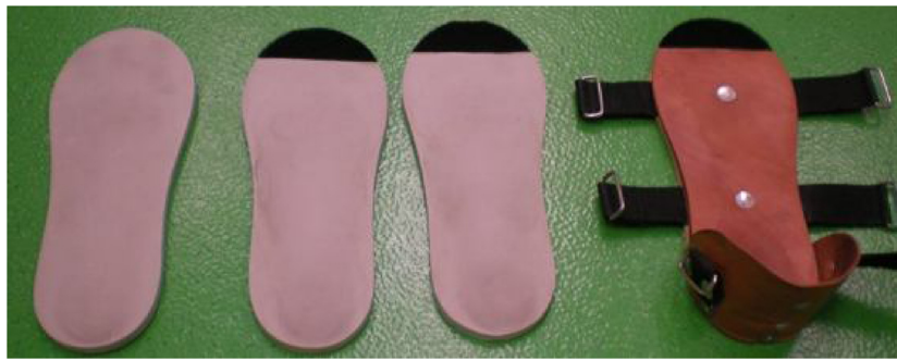
Fig. 1. We constructed a custom sandal in three different sizes. To simulate the different LLIs, three insoles with varying thickness, were added to achieve a maximum LLI of 4 cm.
