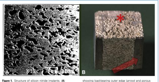
**Figure 1.** Structure of silicon nitride implants. (**A**) Microstructure (×12 Magnification). (**B**) Macrostructure
