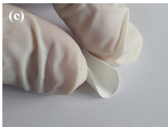
Fig. 3. Microstructure of (a) LTAPO powder, (b) LTAPO-PTFE composite solid electrolyte with 1 M \text{LiPF}_6 in EC/DMC, and image of (c) flexible LTAPO-PTFE composite electrolyte.
