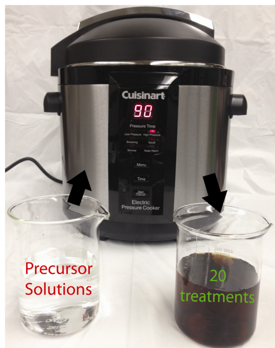
Scheme 1. A domestic electric pressure cooker operating as a hydrothermal reactor for the synthesis of C-dots. The C-dots were synthesized by treating the precursors for twenty consecutive 99-min cycles under the cooker's "high pressure" setting. (No specific endorsement is implied or intended by the use of this particular brand of pressure cooker.)
