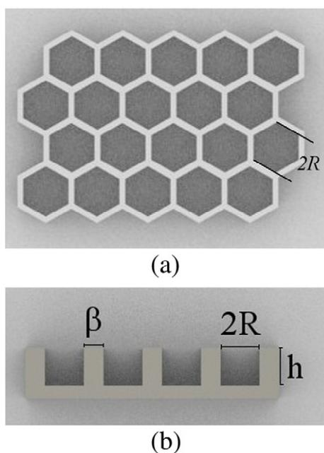
**Fig. 1.** Schematic of the periodic microstructures used. The morphology was composed of hexagonal cavities, shown (a) in top view, and (b) in cross-section.  $R$  is the radius of the inscribed circle,  $h$  the cavity depth, and  $\beta$  the wall thickness between cavities.
