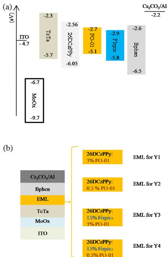
Fig. 1. (a) The energy level diagram of the materials used in this paper, (b) the schematic configuration of yellow OLEDs.
