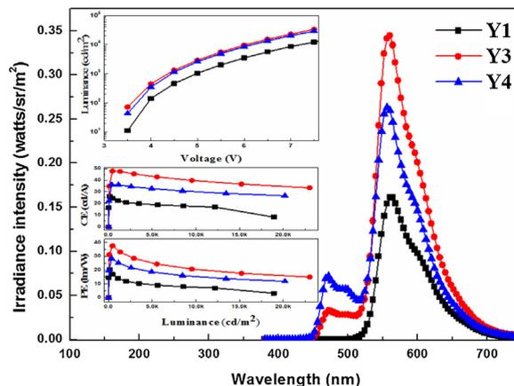
Fig. 2. Absolute irradiance spectra of devices Y1, Y3 and Y4 at the same voltage of 5 V. Luminance versus voltage characteristics (upper inset), CE and PE versus luminance characteristics of devices Y1, Y3 and Y4 (lower inset).
