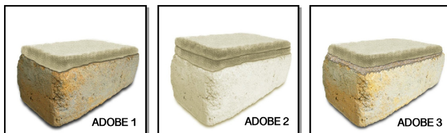
Fig. 1. Application of mortars on adobes.
