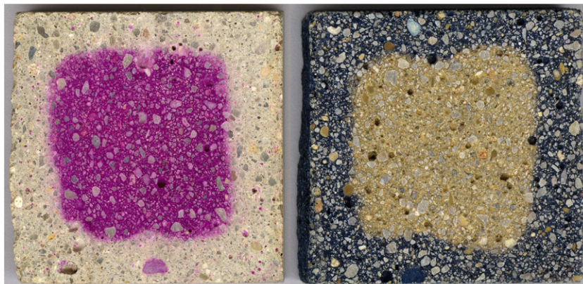
Fig. 1. 4 \times 4 cm mortar sections stained with phenolphthalein (left) and 5 \times 10^{-3} M potassium hexacyanoferrate (II) (right).
