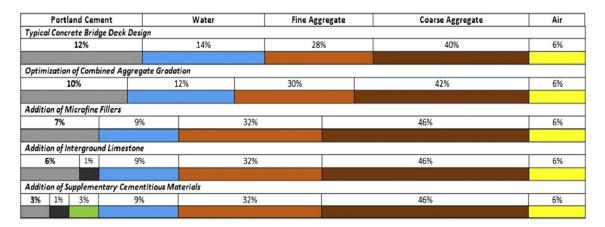
Fig. 1. Illustration of potential reductions in Portland cement content through various methods, including SCM use [9].
