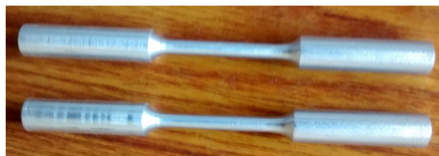
Fig. 1 – Photo of the quasi static tensile specimen of aluminium 7017 alloy.
