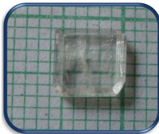
Fig. 2. As grown crystal of 2MIDP.
