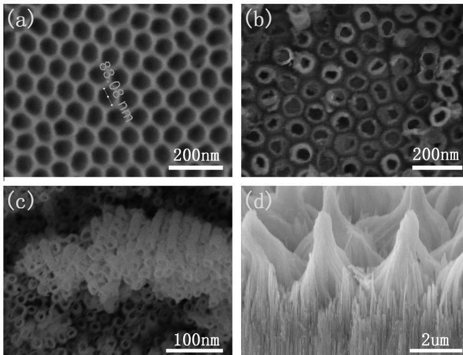
Fig. 2. SEM images of (a) an AAO template, (b) an AAO template filled with PZT nanotubes, (c) free PZT nanotubes, and (d) clustered PZT nanotubes without scaffold of AAO.
