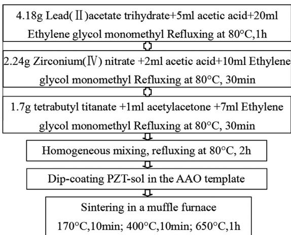
Fig. 1. Flow diagram for the synthesis of the PZT nanotubes.
