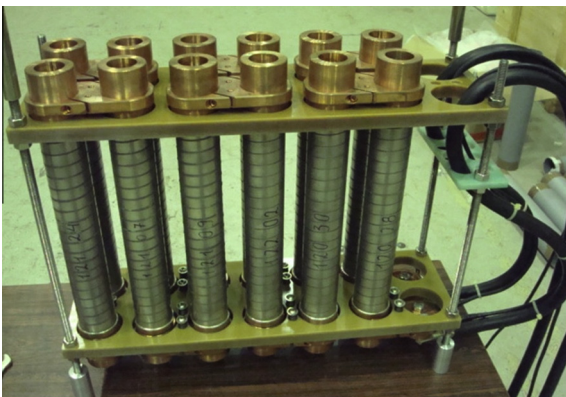
Fig. 1. Twelve tested R-SCFCL components connected in series.
