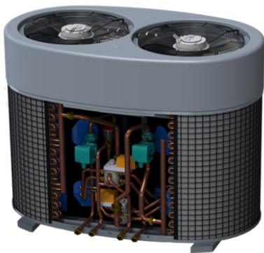
Fig. 1: The hydraulic connections of the Solabchiller® before installation. Connections on the left side are for the cooling circuit of the dwelling and on the right side for the heat source.
