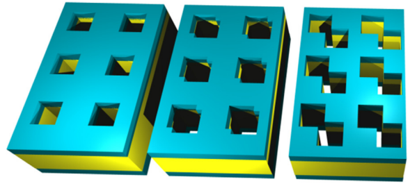
Fig. 1. Fishnet structure (metal-dielectric-metal) without a superstructure array (left) and with a double superstructure with small (middle pattern) and large (right) shift of the basic pattern along both axes.
