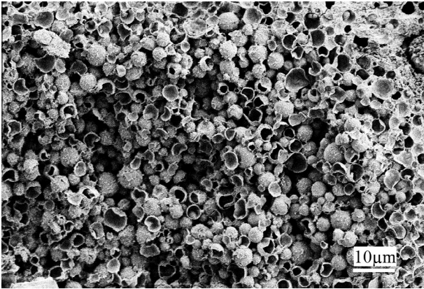
Fig. 1. Breakage of microencapsulated PCMs in cement composites (Li, unpublished work).
