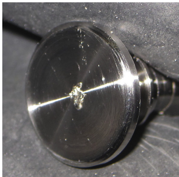
Fig. 2. Photograph of a particle of lithium pressed onto a 13-mm diameter stainless steel SAM stub.
