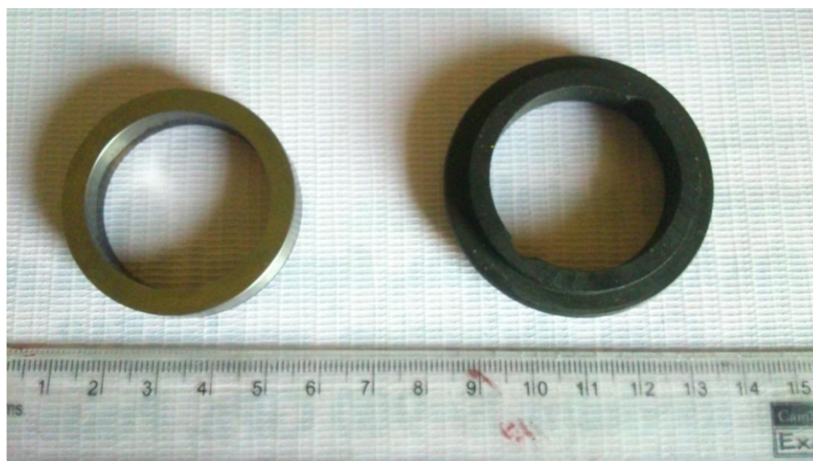
Fig. 1. Photography of stationary seal & rotary seal. [A] Tungsten carbide [B] Resin impregnated carbon.
