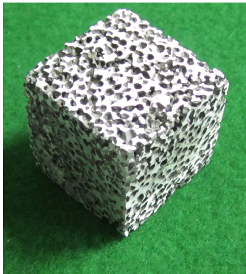
Fig. 1. The open cell AZ31 Mg alloy foam specimen with 1.70 mm \phi (30 mm*30 mm*30 mm).
