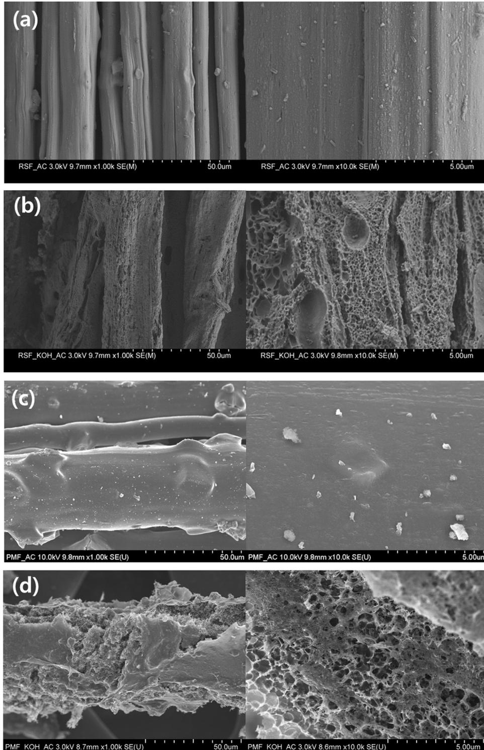
**Fig. 1.** FE-SEM images of the as-prepared products:(a) AC-RSF, (b) RSF-KOH-8M, (c) AC-PMF and(d) PMF-KOH-8M.
