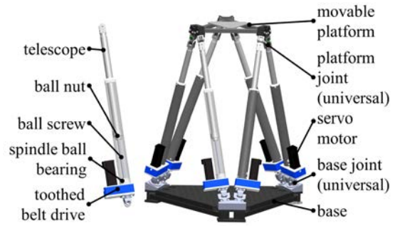
Fig. 2. Structure of the mobile demonstrator (MiniHex).
