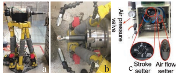
Fig. 1 MQL fitted robotic machining unit. (a) Spindle retrofitted mobile machining (b) MQL mist unit (c) MQL nozzles.
