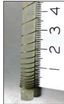
Fig.3 Tool electrode for reverse-tapered hole
