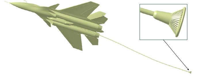
Fig. 1. Geometric model of embarked buddy-refueling aircraft.
